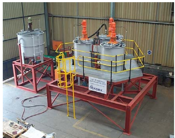
Fig 3: Kemix RIP Pumpcell similar to that being considered at Acoje.
